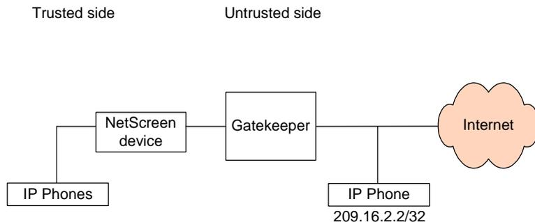
**Figure 2-5** Untrusted Gatekeeper (Transparent or Routed Mode)
