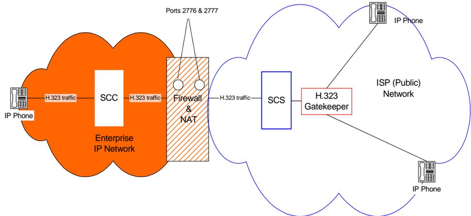
**Figure 4-1** Typical Configuration with Secure Communicator
