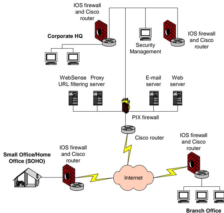
**Figure 2-1** Typical Configuration with PIX and IOS Firewalls
