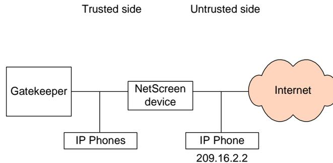
**Figure 2-3** Trusted Gatekeeper (Transparent or Routed Mode)
