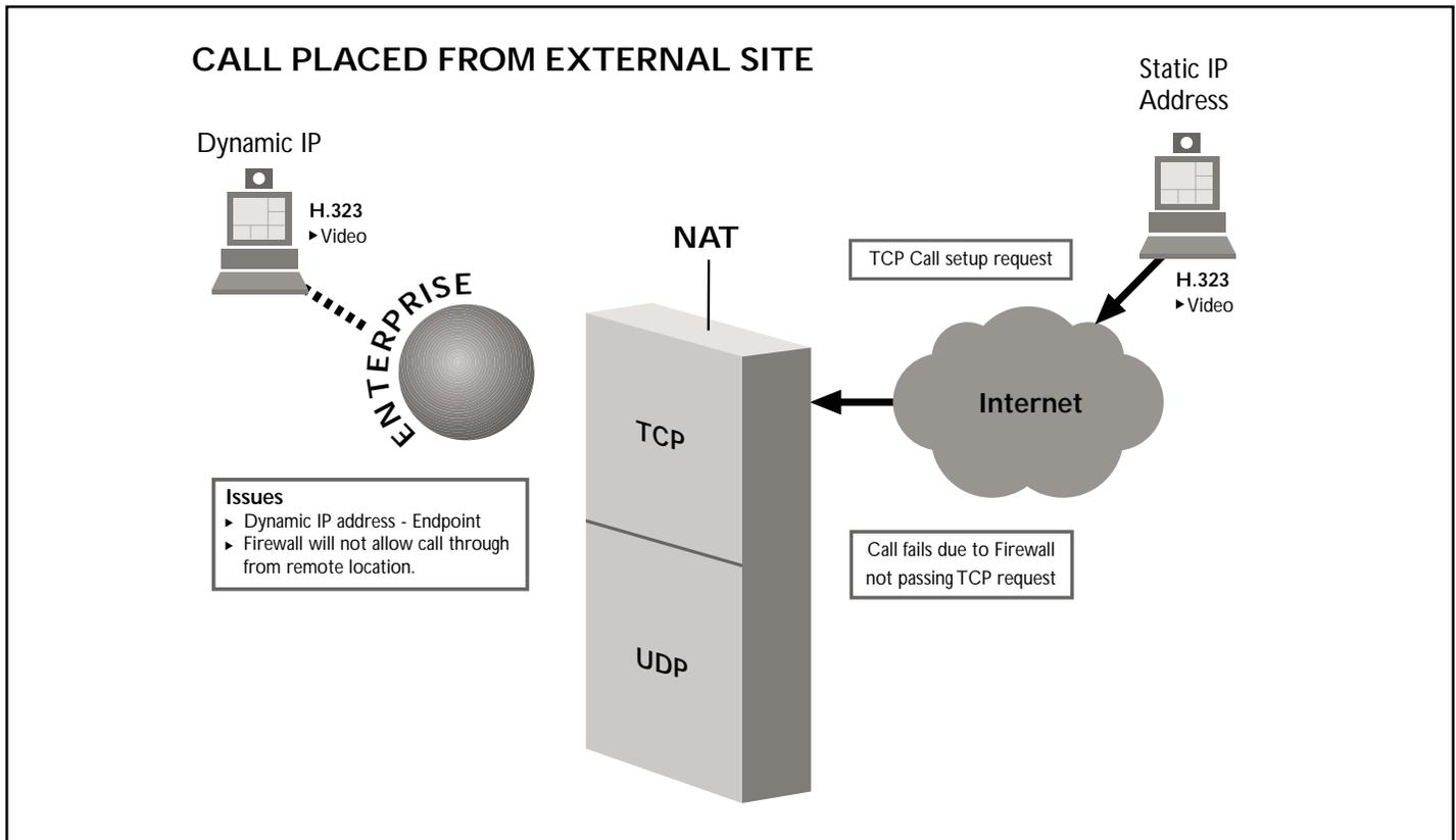
Even when an H.323-savvy NAT device or firewall is in place, typical solutions on the market today will terminate the media streams when the TCP H.225 channel is closed. In addition, the H.323-compliant NAT/PAT devices currently available do not support multicast because the network behind them appears as a single address preventing the router from detecting the identity of multicast requests received from inside the network.
