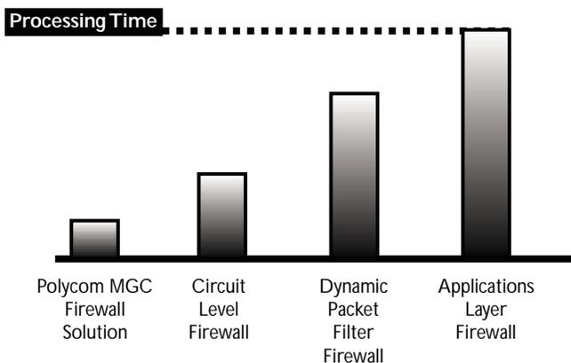
Application layer firewalls also implement the broadest set of security data checks, which increases the processing time required. Throughout the industry, application layer firewalls are generally considered to provide the best security.
