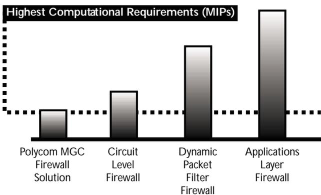
However, because a circuit level firewall does not perform extensive security checks, other than whether a network packet is associated with a valid connection, it can (and often does) perform faster than a packet filter firewall that contains a large set of accept and deny rules.
